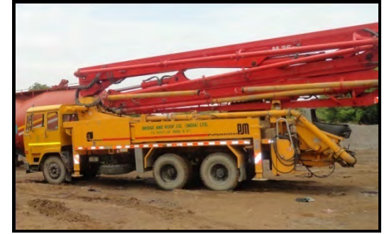
Concrete Placer Boom Pump
