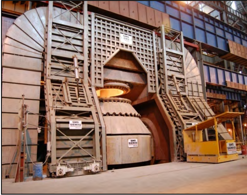
LD Converters for Visakhapatnam Steel Plant 6.3 MTPA Expansion Project of Rashtirya Ispat Nigam Ltd.
